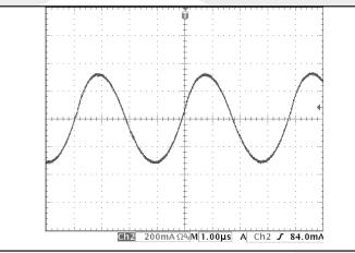
**Figure 9:** Input terminal current ripple,  $i_{C}$ , at full rated output current and nominal input voltage with SynQor MCOTS filter module (200 mA/div). Bandwidth: 20MHz. See Figure 17.
