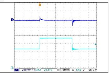
*Figure 12:* Output voltage response to step-change in input voltage (1000V/ms). Ch 1: Vout (200mV/div), Ch 2: Vin (20V/div).
