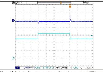
**Figure 11:** Output voltage response to step-change in load current (50%-75%-50% of lout(max);  $dI/dt = 0.1 A/\mu s$ ). Load cap: 1  $\mu$ F ceramic and 15  $\mu$ F tantalum capacitors. Ch 1: Vout (100mV/div), Ch 2: lout (5A/div).
