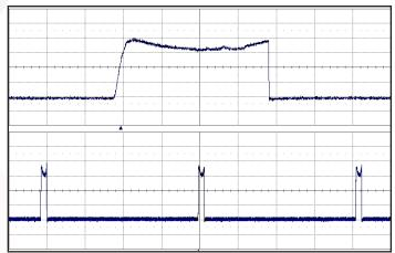
**Figure 18:** Load current (10A/div) as a function of time (1ms/div and 50ms/div) when the converter attempts to turn on into a 10 m $\Omega$  short circuit.
