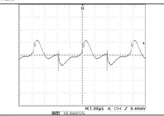
**Figure 10:** Output voltage ripple, Vout, at nominal input voltage and rated load current (10 mV/div). Load capacitance:  $1\mu F$  ceramic capacitor and  $10\mu F$  tantalum capacitor. Bandwidth: 10 MHz. See Figure 17.
